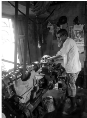
It's a Lathe Machine to Prepare the different parts.
